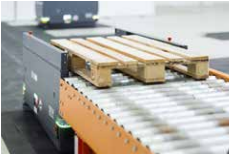
Plate transfer with roller conveyor The integrated longitudinal conveyor allows load to be transferred to a station on both sides.
