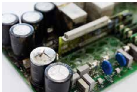
Reforming to prevent capacitor explosions
