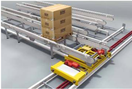
Pallet transfer carriage
