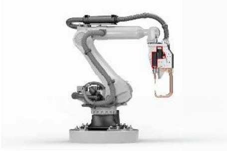
Welding tongs e.g. in the automotive industry
