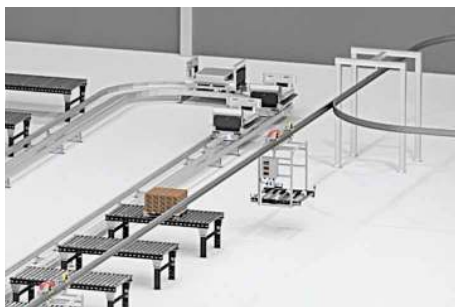
Floor track system (FTS)
