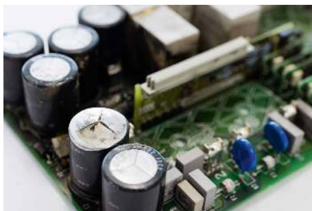
Forming to prevent capacitor explosions
